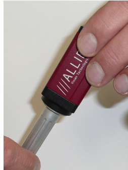
Figure 4: Removing IR cut filter/protection glass using special tool (E902001)
